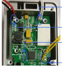
**OUTX (white):** The output of the relay is connected with the electromagnetic switch, used to control the door.
