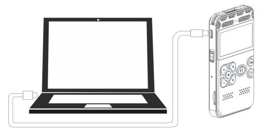
Connect the Recorder to the PC via the USB cable.
