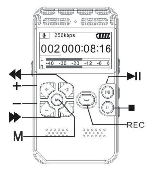
Press the "Record button" in "REC" to start recording in the stop mode, the operation indicator light flashes
