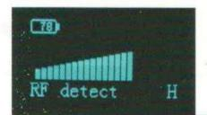
This function is mainly used to detect all kinds of GPS locators, WiFi cameras, eavesdroppers issued by the electromagnetic wave signal. OK key can be used to adjust the detection sensitivity. Users need to turn off their mobile phones, routers in the environment and other strong interference devices to detect.
